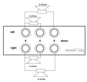
Figure 2: model i84 speakers connection
