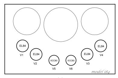
Figure 1: model 184 tube layout
